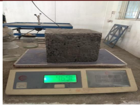
Figure 4: Water absorption test
